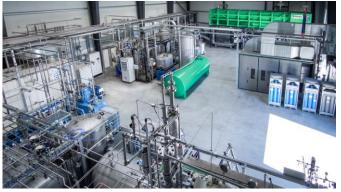
Fraunhofer large-scale demonstrator for the decentralised conversion of sewage sludge into petrol and diesel fuel, and the production of »green« hydrogen.
