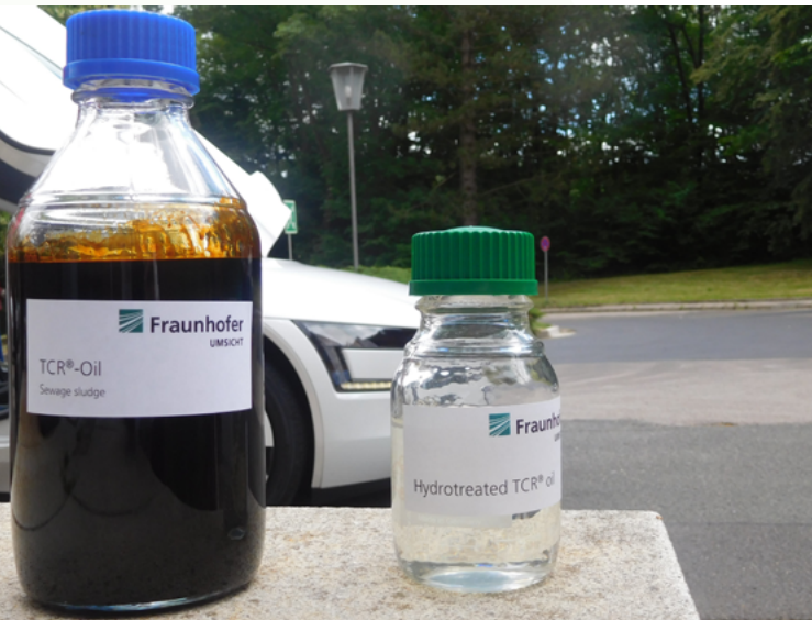
Figure 8: Samples of TCR-oil from sewage sludge and upgraded TCR-oil. Credit: TO-SYN-FUEL project.
