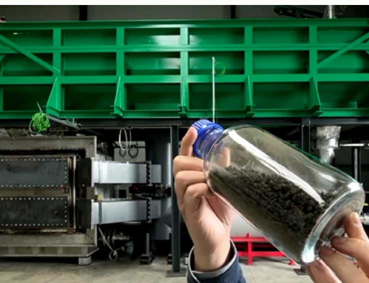
Figure 3: Dried sewage sludge feedstock. Credit: TO-SYN-FUEL project.
